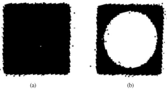
Fig. 5. Validation experiments with stagnant fluid. (a) 5 mm square channel; (b) 5 mm square channel with \varnothing 4 mm round channel inserted. MRI parameters as in Fig. 4, except image matrix 192 \times 192 , field of view 15 mm, repetition time 1 s, no. averages 4, no. echoes 32, slice thickness 4 mm, first echo time 6.0 ms, echo time in train 5.4 ms, total measurement time 13 min.
